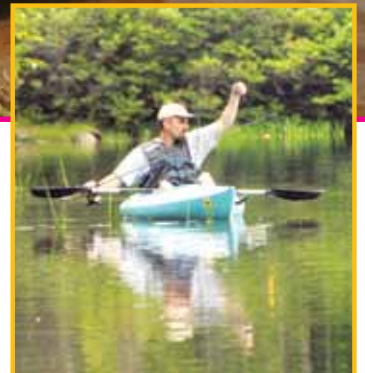
Fishing kayak models have generous width and stability to handle the angling paddler's increased body movements not only when casting and reeling, but also when fighting fish.
